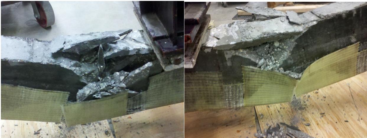
Figure 15—FRP Rupture of Shear Reinforcement and Concrete Crushing of the Beam R4 with 7-ft NSM rebars
