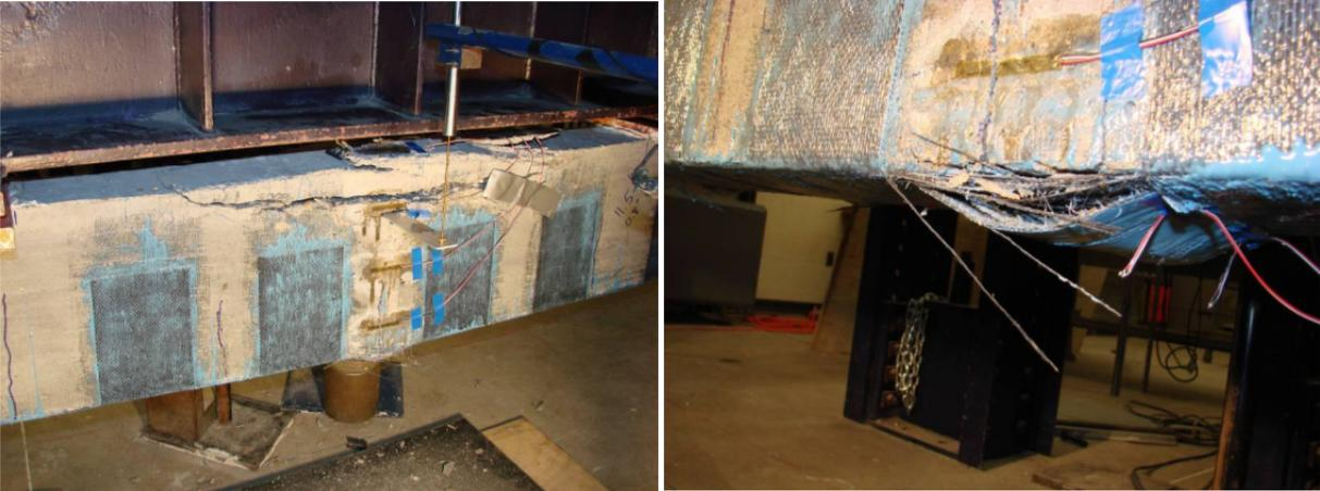
Figure 13—Concrete Crushing followed by CFRP Rupture in Beam R3
