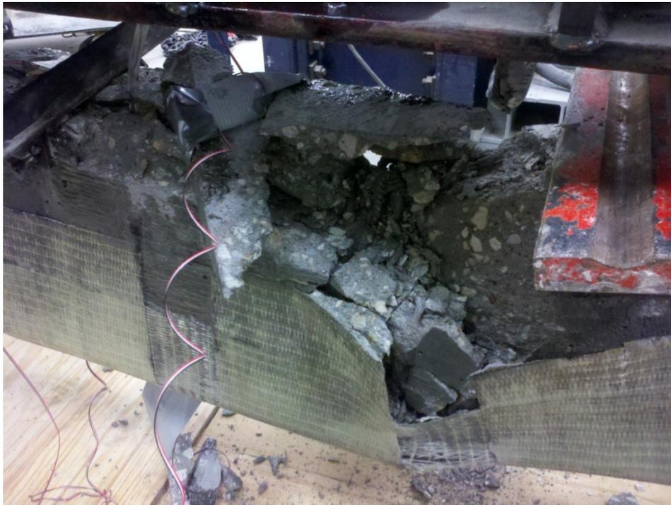
Figure 11—Concrete Crushing of the Beam R2 with the Full Length NSM rebars
