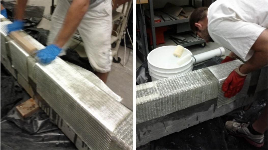
Figure 8—Applying U-Wraps to Beam R4
