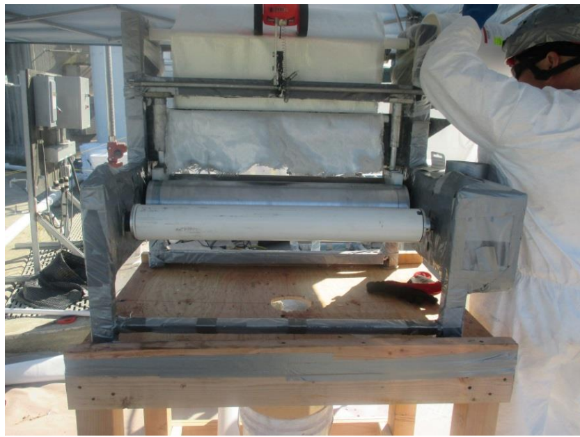
Figure 3. Glass fabric being saturated with a two-part 100% solid epoxy using a mechanical saturator
