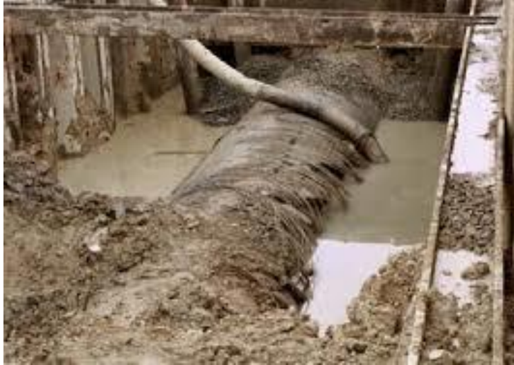
Figure 2. Failed section of PCCP
