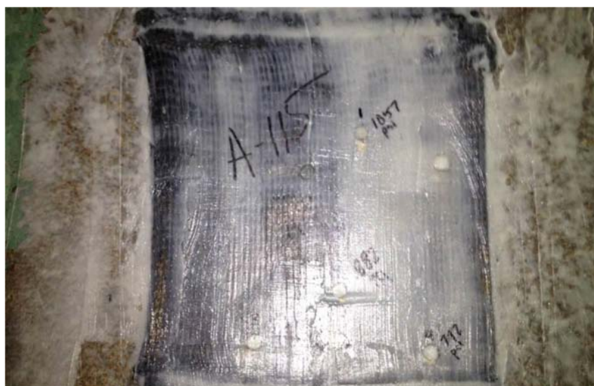
Figure 9. ASTM D4541 bond test typical patch
