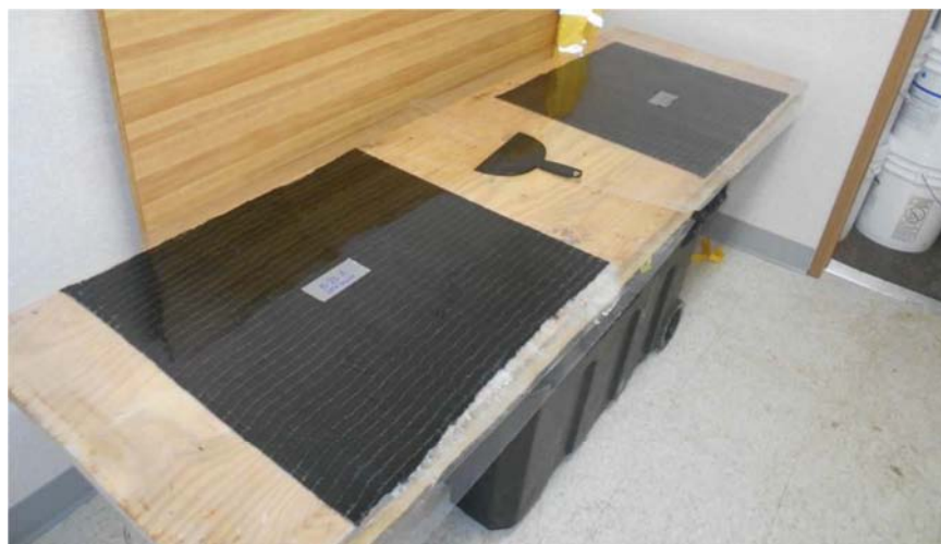
Figure 10. ASTM D3039 Tensile Testing panel preparation
