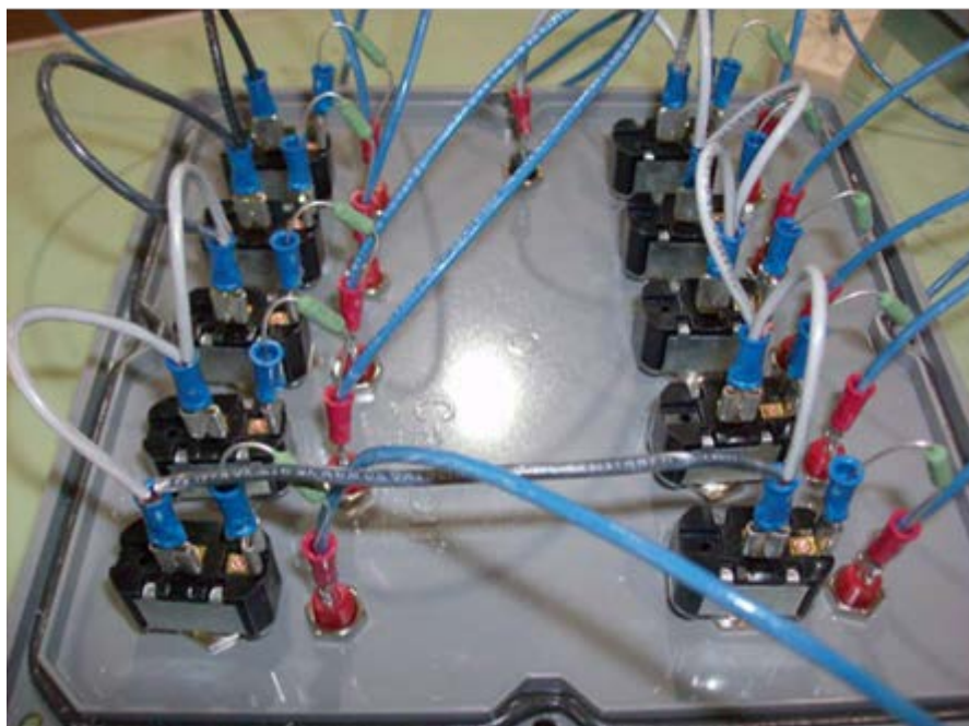
Figure 7 – Wiring in NEMA 4X Box for a ten circuit system for Configuration B test slab.
