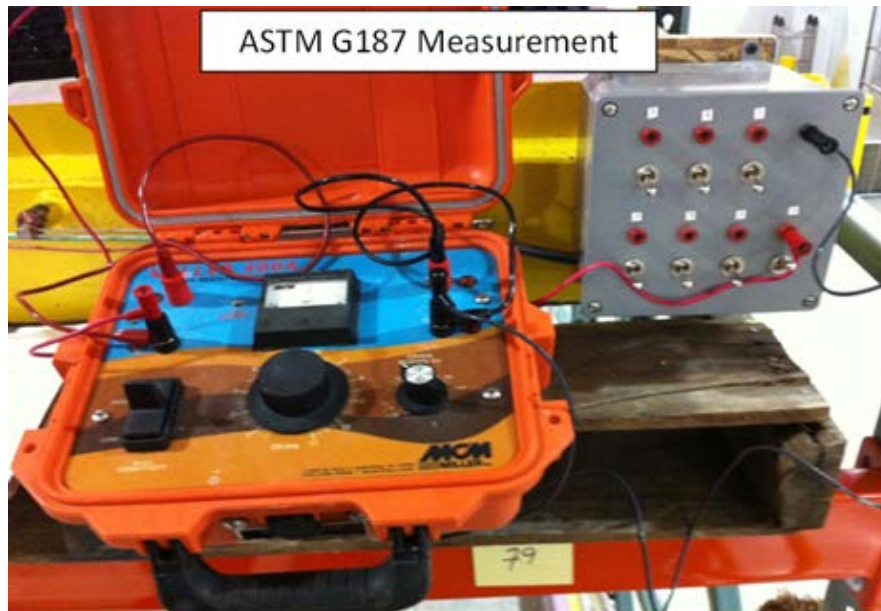
Figure 13 – Example for measuring mat-to-mat resistance.
