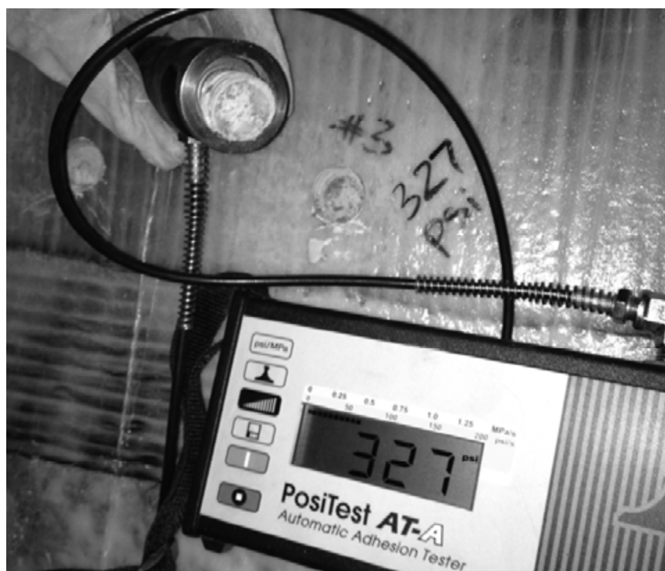
Figure 9. Adhesion test equipment used for ASTM D4541 test
