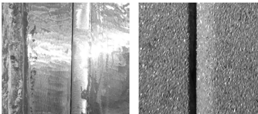
Figure 8. Close up of prepared steel substrate in joint region of PCCP with grinder (left) and sponge blasting (right)
