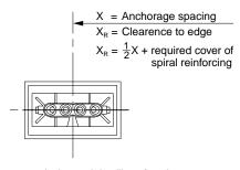
For proper design and detailing of anchorage zones and related reinforcement, refer to the VSL Publication "Detailing for Post-Tensioning". The arrangement shown here is common for slabs in buildings.
