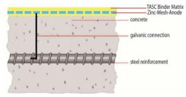
encompass the zinc mesh. The binder forms a matrix with excellent adhesion to concrete surfaces, with a volumetric porosity of >35%, high ionic conductivity and high durability.
