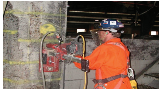
Figure 9 – Concrete Core Sampling (ASTM C42) using a wet rotary diamond tipped core-drill.
