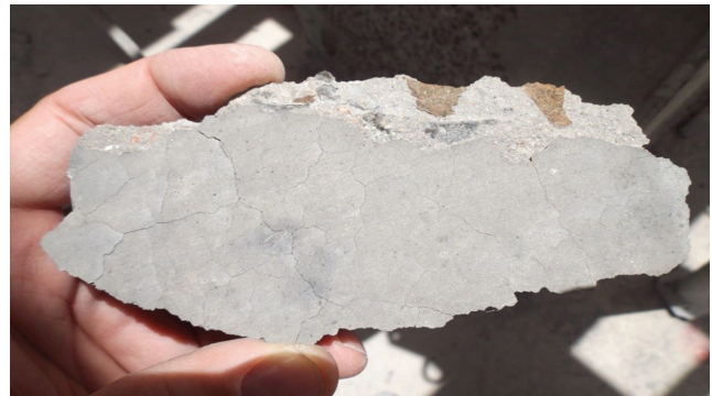
Figure 2 – Spalled concrete piece that jettisoned off of a concrete Column member which was only 3 days-old at the time of the fire event due to “green concrete conditions”. Significant moisture in near surface regions phase-changed the pore moisture from liquid water to steam. The steam formation pressurized the denser concrete surface creating internal separations approximately \frac{3}{4} ” (19mm) in thickness, roughly the size of the coarse aggregate in the concrete mix.
