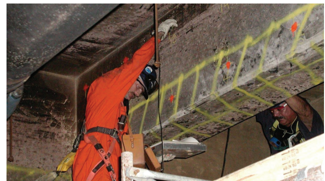
Figure 6 – Ultrasonic Pulse Velocity Testing (ASTM C597) on a fire-damaged conventionally reinforced concrete beam. Note both sides of the structural member need to be accessible. Mechanical hammer sounding (ASTM D4580) revealed delaminated conditions along the beam bottom.
