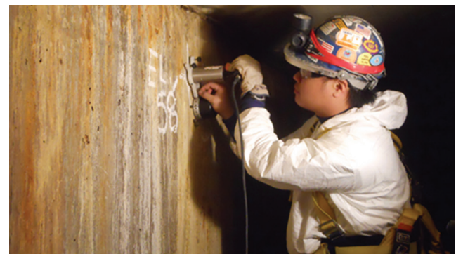
Figure 7 – Impact Echo Testing (ASTM C1383) on a fire-damaged interior Silo Wall which provided information on internal cracking and relative soundness of the concrete from single side access.
