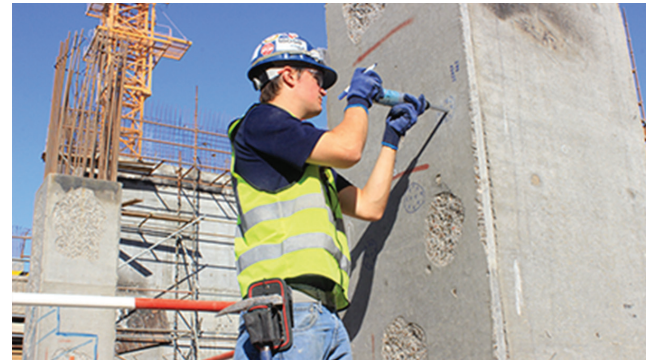
Figure 5 – A Technician employing a Rebound Hammer (ASTM C805) to a fire-affected Column surface to establish surface hardness consistency.
