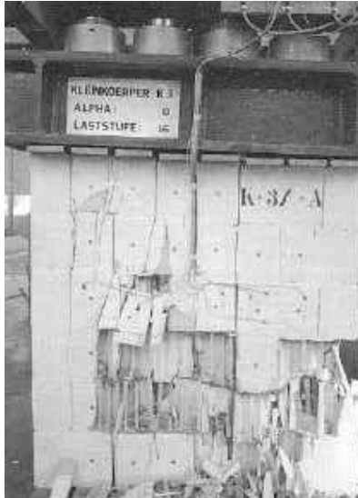
a) Compressive failure of units
