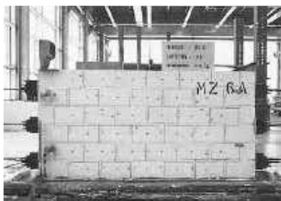
d) Tensile failure along joints
