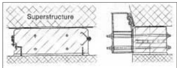
Fig. 14: Temporary sliding bearing with lateral guide
