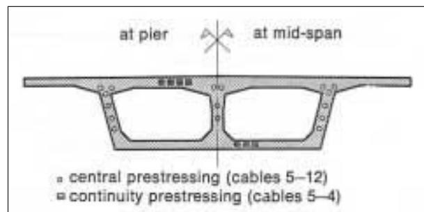
The unusual arrangement of the cables was due to the constraint that the cross-section dimensions of the original design had to be retained. The use of small cables for the eccentric prestressing had, however, the advantage that the stressing buttresses were very small and a small, light jack, very easy to use for overhead work, could be used for stressing.
