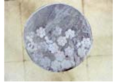
Fig. 3: Properly grouted tendon section
