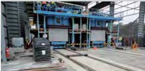
Two match-cast pier moulds in operation
