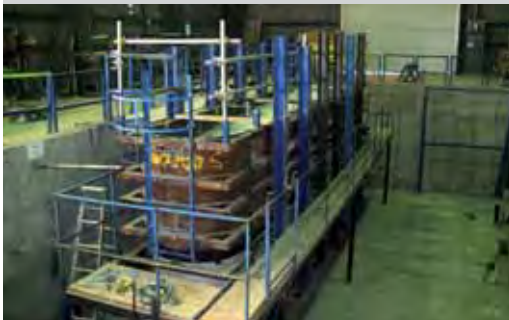
Match-cast pier mould in operation
