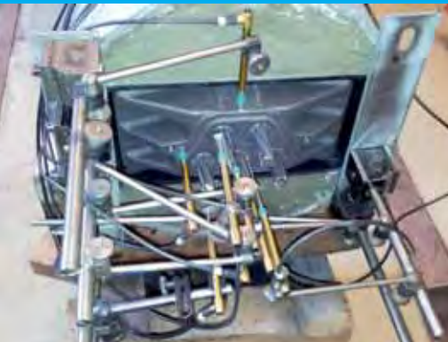
Resistance to static load: a 6-5 anchorage with measuring equipment during static testing
