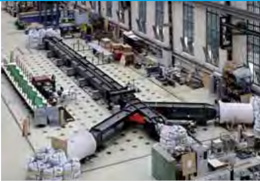
Machine for small radius saddle testing, installed in the laboratory of the technical university of Berlin
