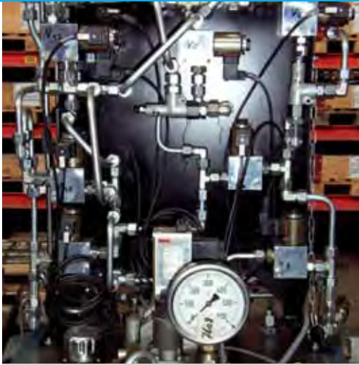
Hydraulic circuitry with 12 valves added to a standard heavy lifting pump unit.
