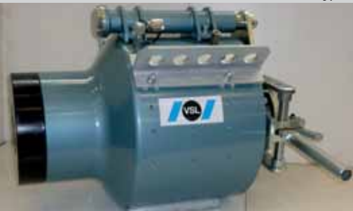
Mid-range size stressing jack ZPE980, capacity: 980tons at 600bar, designed to stress up to 31 numbers of 0.6" strands
