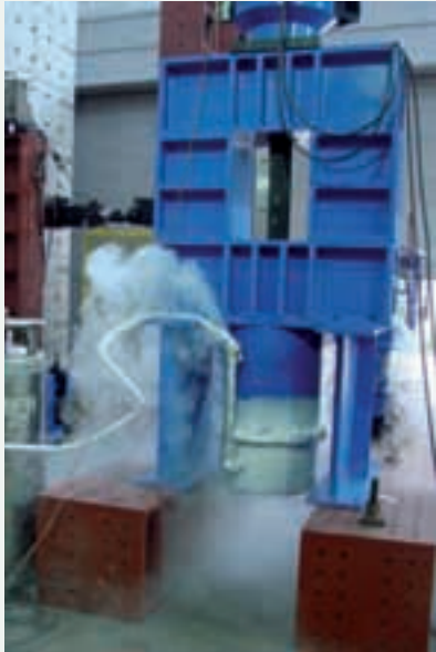
Cooling of dead end anchorage by injecting liquid nitrogen N2 into cryogenic chamber during 10 cycles loading, Daewoo Laboratory, Seoul
