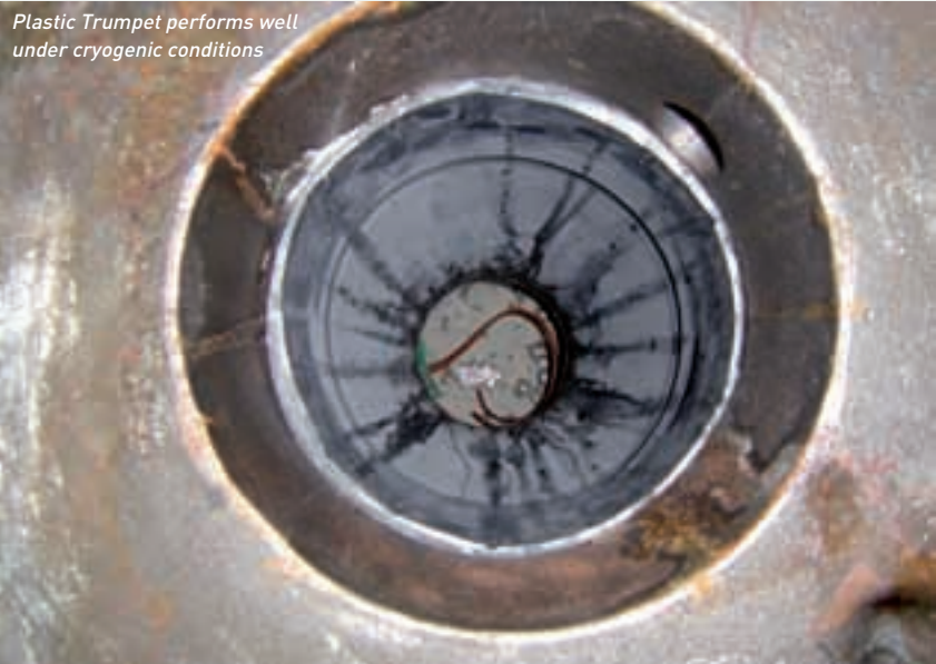
Cooling of dead end anchorage by injecting liquid nitrogen N2 into cryogenic chamber during 10 cycles loading, Daewoo Laboratory, Seoul
