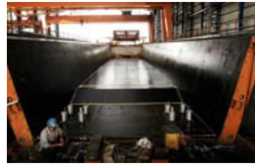
7 Strand preparation. Cleaning of the strand coupler attached to the coupling strands. After cleaning the strands, the rebar cage will be lifted into the mould and the couplers connected to the strands in the cage.
