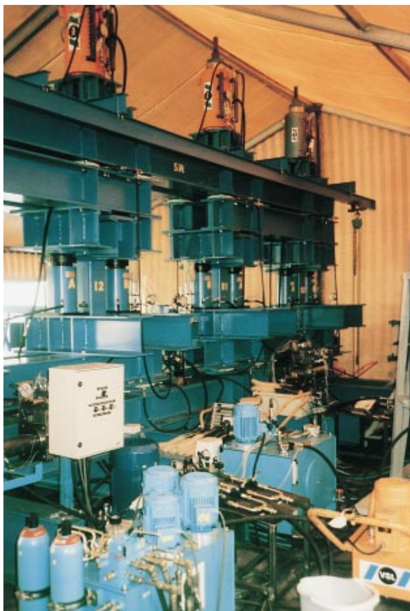
Partial view of test rig for vertical B jack system
