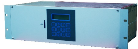
TRIM unit with microcontroller housed in a 19" rack assembly for inclusion within TR enclosure
