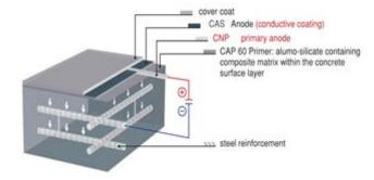
high durability, high weathering resistance (UV-resistance, frost resistance, freeze-thaw salt resistance\*) and compatibility with most acrylic, PU and epoxy based paint and coating systems. The CAS composite coating is applied on concrete surfaces impregnated with the CAP60 primer. The CAP60 primer is especially designed for the CAS coating, enhancing adhesion to the concrete surface and promoting ionic transport across the concrete overlay.
