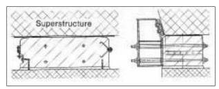
Fig. 14: Temporary sliding bearing with lateral guide
