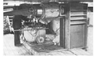
Fig. 13: VSL-jacks with suporting structure
