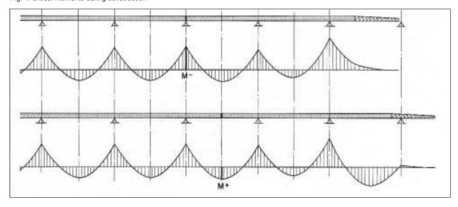
Fig. 4: critical moments during construction
