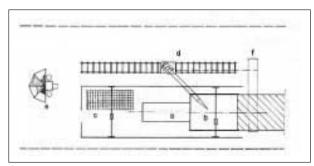
For a box-section structure, construction is usually carried out in two phases: in the rear part of the fabrication area, the bottom slab is cast, while the webs and deck slab are cast in the forward part. Consequently, there are two formwork units (fig. 9). The rear formwork, where accuracy is of especial importance so that the
