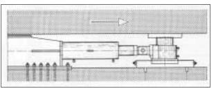
This type of sliding equipment can be used where the applied force is sufficiently large in relation to the sliding force required.
