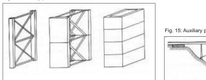
can with advantage be built up from prefabricated components, and their subsequent removal therefore presents no special problems. This also permits a certain amount of reuse. Some examples of auxiliary pier designs may be seen in fig. 15.
